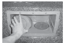
Install Eco Pur filter on left side.
