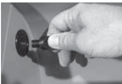
Air Bleed Valve
